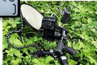
ABOVE: A typical set-up for a flower shot, showing a Wimberley Plamp, holding the white reflector in place.
